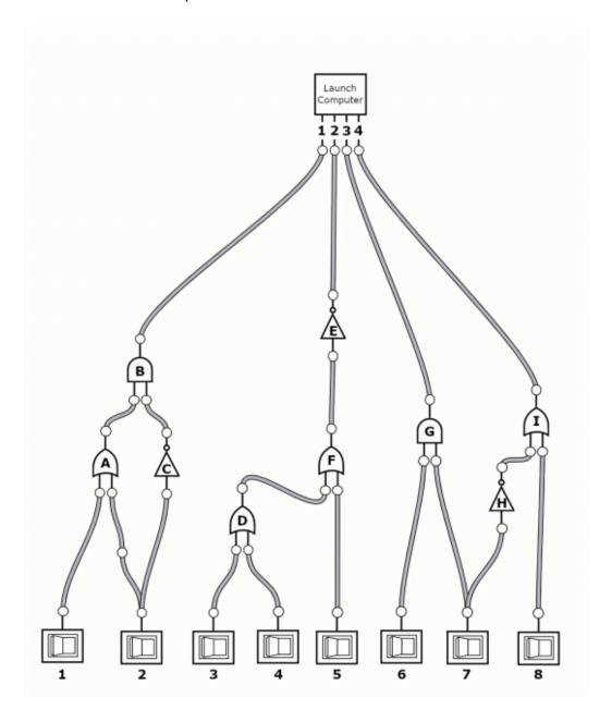
The circuit uses three types of logic gates that may output power depending on what inputs they receive:
